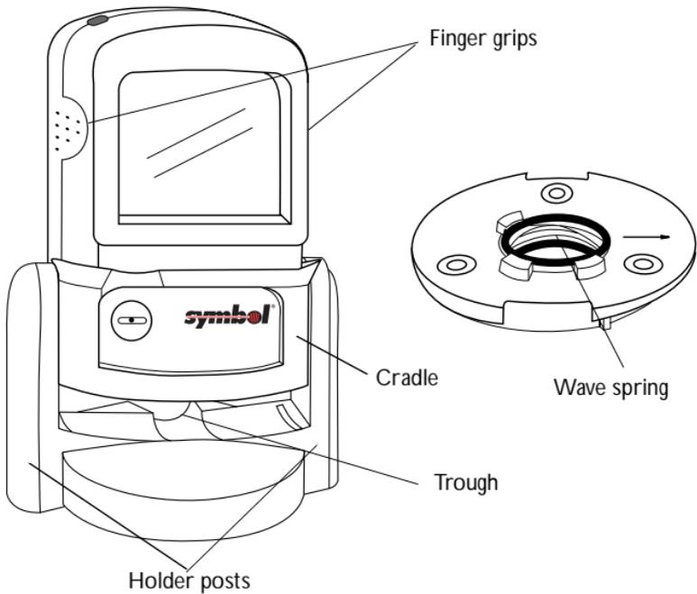
Figure 1-2. Parts of the LS 9100
