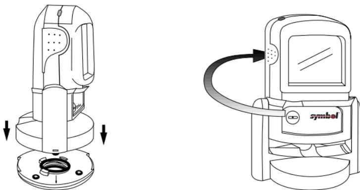
Figure 1-4. Placing Scanner onto Mounting Plate
