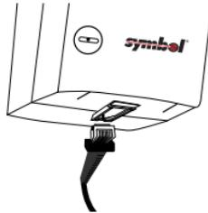
Figure 1-11. Connecting Cable to Scanner
