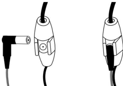
Figure 1-10. Inserting Power Supply
