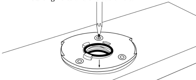
Figure 1-5. Marking Mounting Holes
