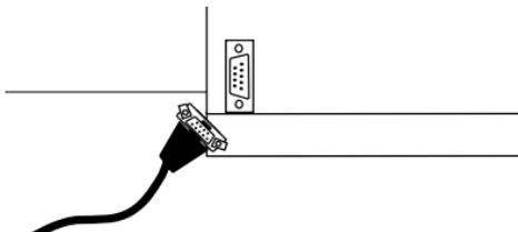
Figure 1-9. Connecting Cable to the Terminal
