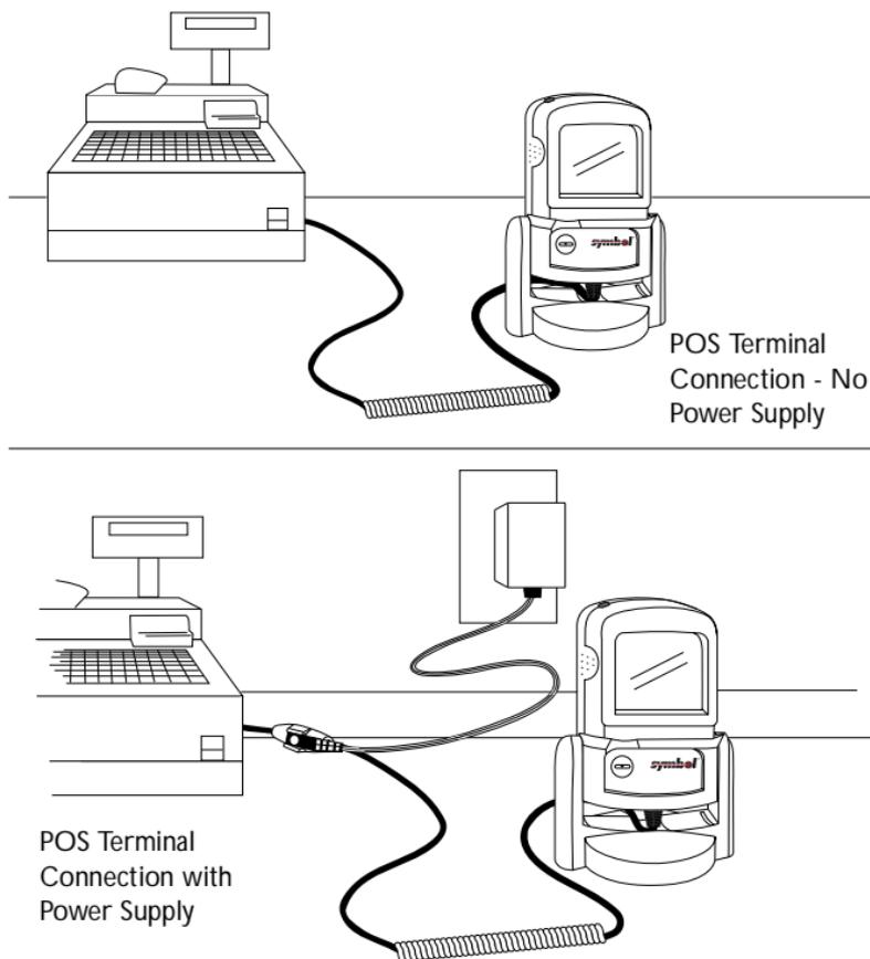
Figure 1-8. Scanner Configurations
